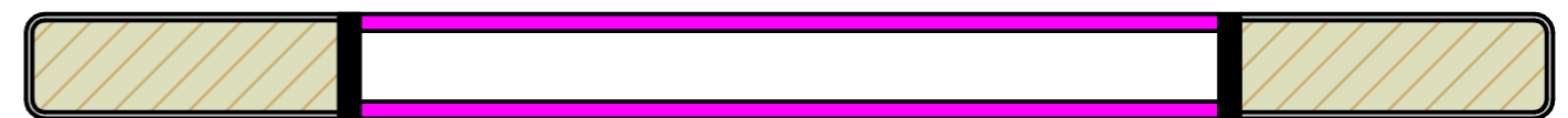
Option 4 Pre-made Flush Glazed Panel Silicon Bead (Option to also use thinner panels/panels with integral blinds with silicon bead, bolection bead or stainless steel surround)
