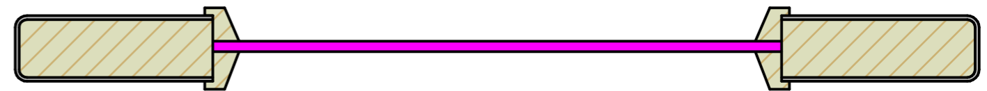
Option 2 Glazed Vision Panel Bolection Bead - Finished as hardwood or wrapped
